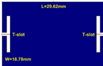
**Fig. 6.** The layout of the studied microstrip patch antenna with two T- notches.
