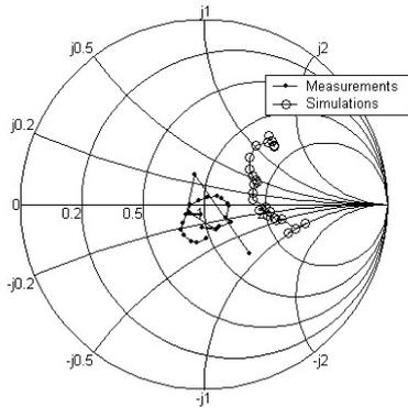
Fig. 10. The Smith chart of the input impedance – model 1.
