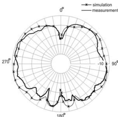
Fig. 16. The elevation cut of radiation pattern @ 2100MHz.
