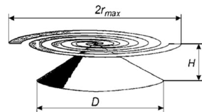
Fig. 1. Combined spiral-discocone antenna.
