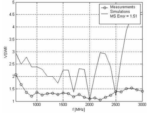
Fig. 12. The comparison of VSWR obtained from simulations and measurements for model 2.
