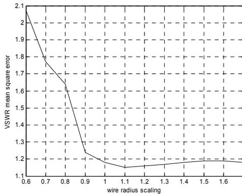
Fig. 11. VSWR error vs. wire radius scaling factor in model 1.
