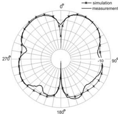
Fig. 15. The elevation cut of radiation pattern @ 1000MHz.
