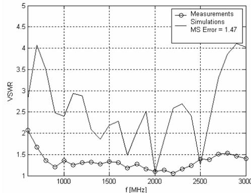
Fig. 14. The comparison of VSWR obtained from simulations and measurements for model 3.
