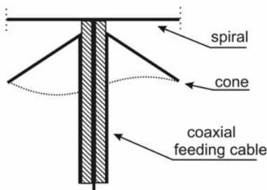
Fig. 2. The feeding of combined spiral-discone antenna.
