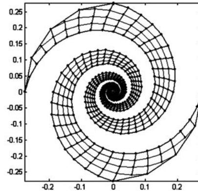
Fig. 3. The wire-grid model of the spiral component of the antenna.
