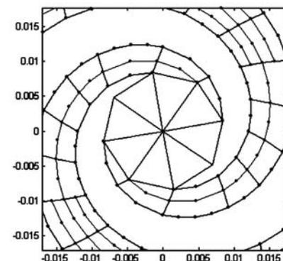
Fig. 4. The layout of wires at the excitation point of the spiral.
