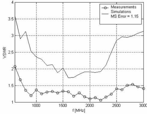
Fig. 9. The comparison of VSWR obtained from simulations and measurements for model 1.
