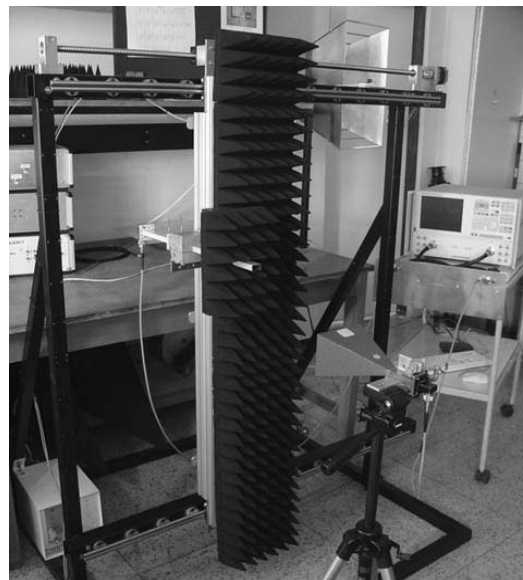
Fig. 4. Measurement setup in the case of horn antenna.
