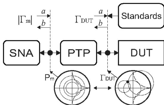
Fig. 1. Block structure of a measurement system with PTP.
