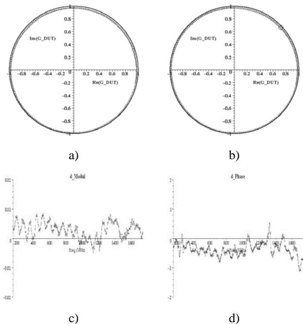
**Fig. 9.** Comparison of reflection coefficient measured on VNA and via PTP. The DUT is formed as Long Line and the short. Frequency range 190-1700 MHz.
