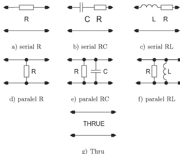
Fig. 2. Seven different internal PTP states realized by simply passive RLC structure.
