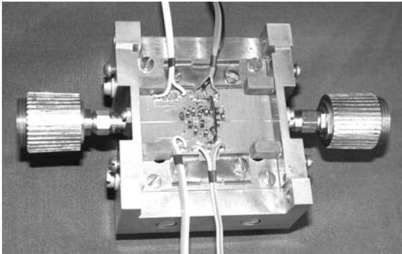
Fig. 4. Test fixture with PTP that was used for verification.
