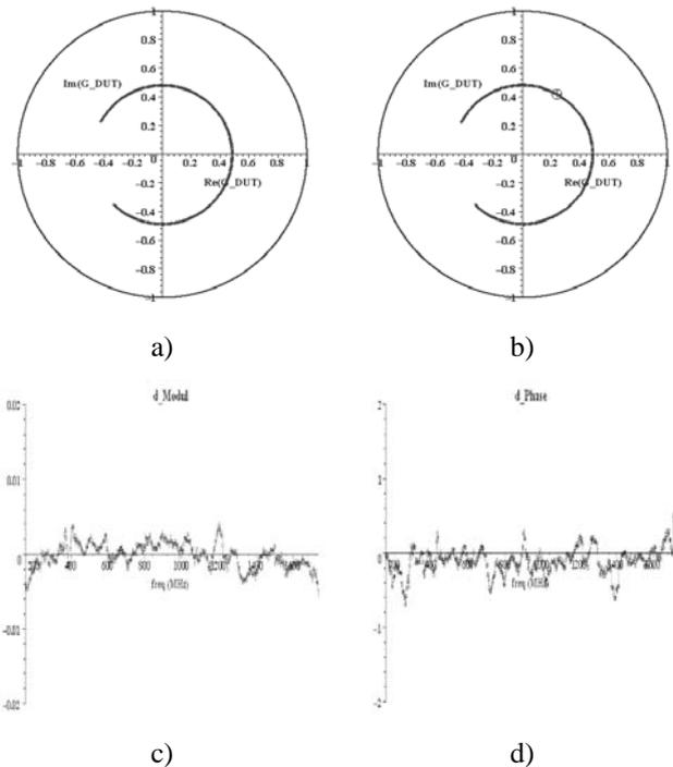
Fig. 8. Comparison of reflection coefficient measured using VNA and via PTP. The DUT is formed as 3-dB attenuator and the short. Frequency range 190-1700 MHz.
