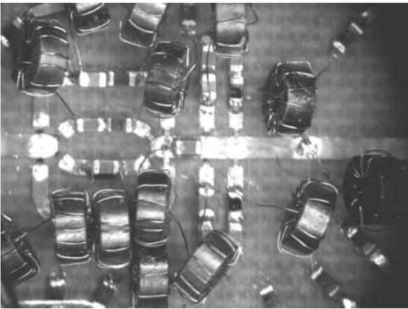
Fig. 3. Detail of the microstrip PTP realization.
